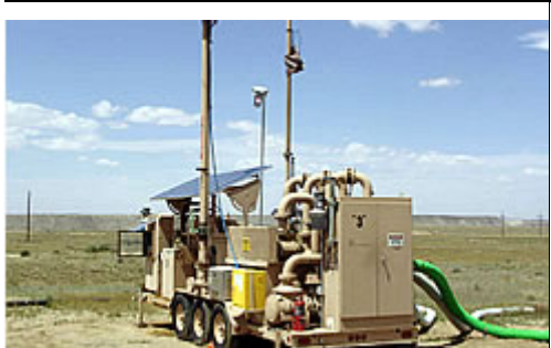
Mechanised drainage unit removes excess methane from the caved area (gob) behind the longwall
